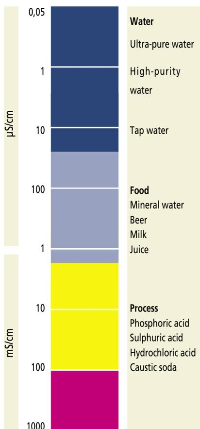
The conductivity meter measures the electrical conductivity of the ions in a solution. To do this, it applies an electrical field between two electrodes and measures the electrical resistance of the solution. To prevent changes occurring in the substances, or the deposit of a layer on the electrodes, etc., alternating current is used.
